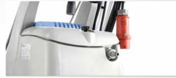
Always on the safe side: A float regulates the water inflow and prevents damage to the pump due to a lack of water.
